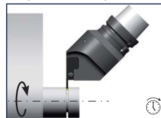
GLM 45° left hand basic tool holder + left hand cartridge
