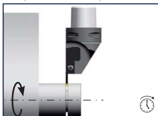
GLM 0° left hand basic tool holder + left hand cartridge
