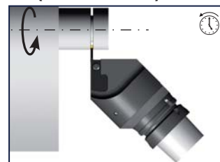
GLM 45° right hand basic tool holder + right hand cartridge
